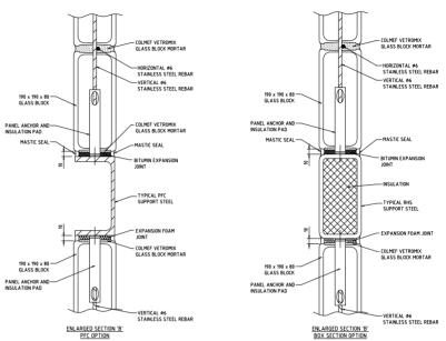
TYPICAL SUPPORT STEELWORK IS ONLY REPRESENTATIVE AND IS TO BE DESIGNED AND CONFIRMED BY ARCHITECT AND STRUCTURAL ENGINEER TO SUIT SPECIFIC PROJECT.
